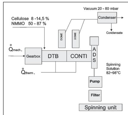
Fig. 2 P & F diagram of the List cellulose solution-step
