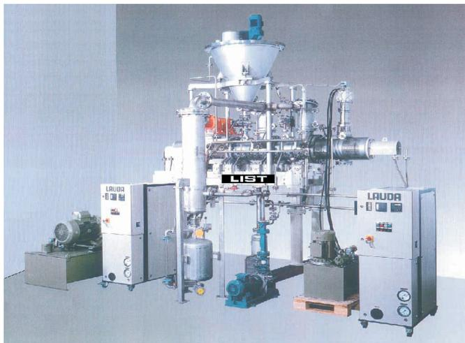
Fig. 1 Dissolving unit of the 3rd generation
