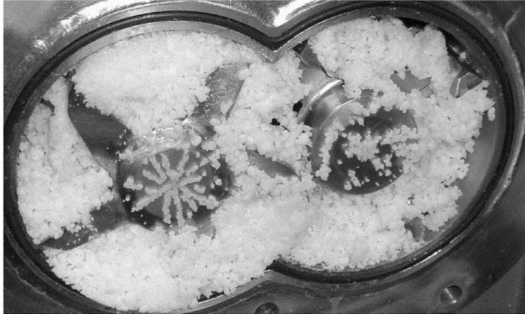
**Figure 3:** Rubber Crumble Formation in Finisher
